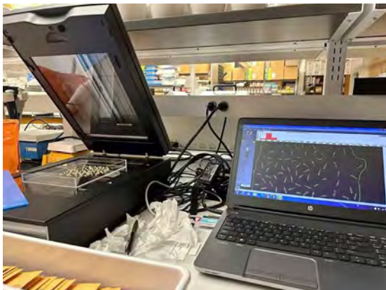
Measuring the chalk area in rice grains using WinSeedle™ instrument.
